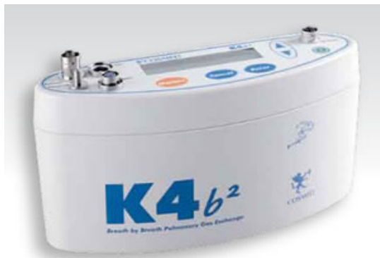
Figure 2: Portable metabolic cart used as the criterion measure to measure energy expenditure in the subjects
